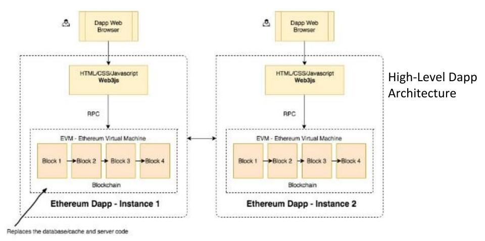
Figure 4.1: High-level DApp architecture, Source: Mahesh Murthy, medium.com
