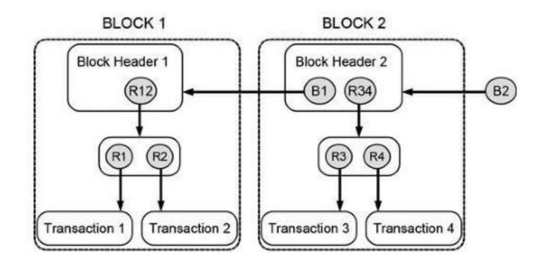
A simplified blockchain-datastructure containing four transactions
