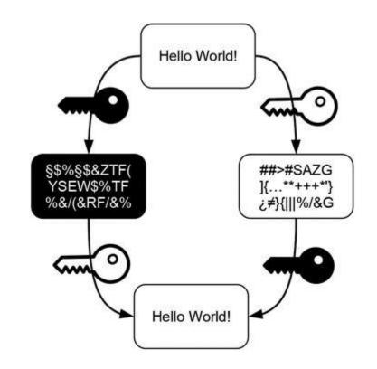
*Figure 12-3.* Schematic illustration of asymmetric cryptography
