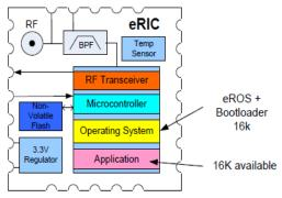
Figure 1 eRIC Transceiver Block Diagram
