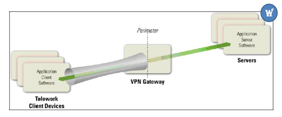
Figure 2-1. Tunneling Architecture
