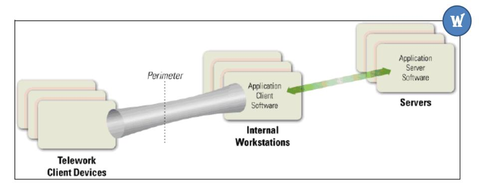
Figure 2-3. Remote Desktop Access Architecture
