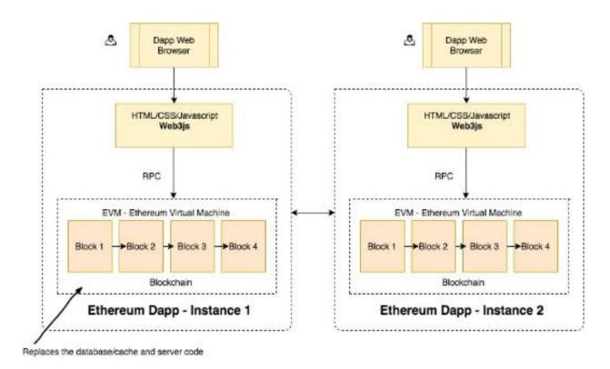
Figure 4.1: High-level DApp architecture, Source: Mahesh Murthy, medium.com
